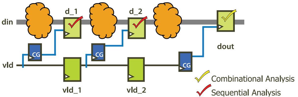
Figure 3: PowerPro employs Observability-Based Sequential Clock Gating
