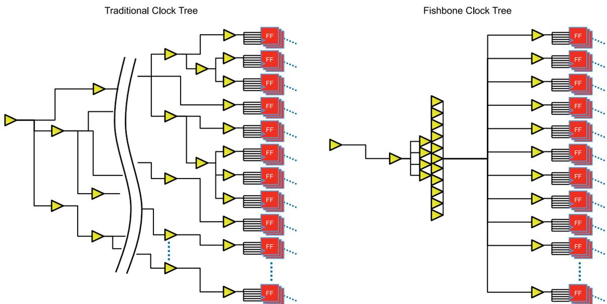
Figure 1: Clock tree methodology comparison
