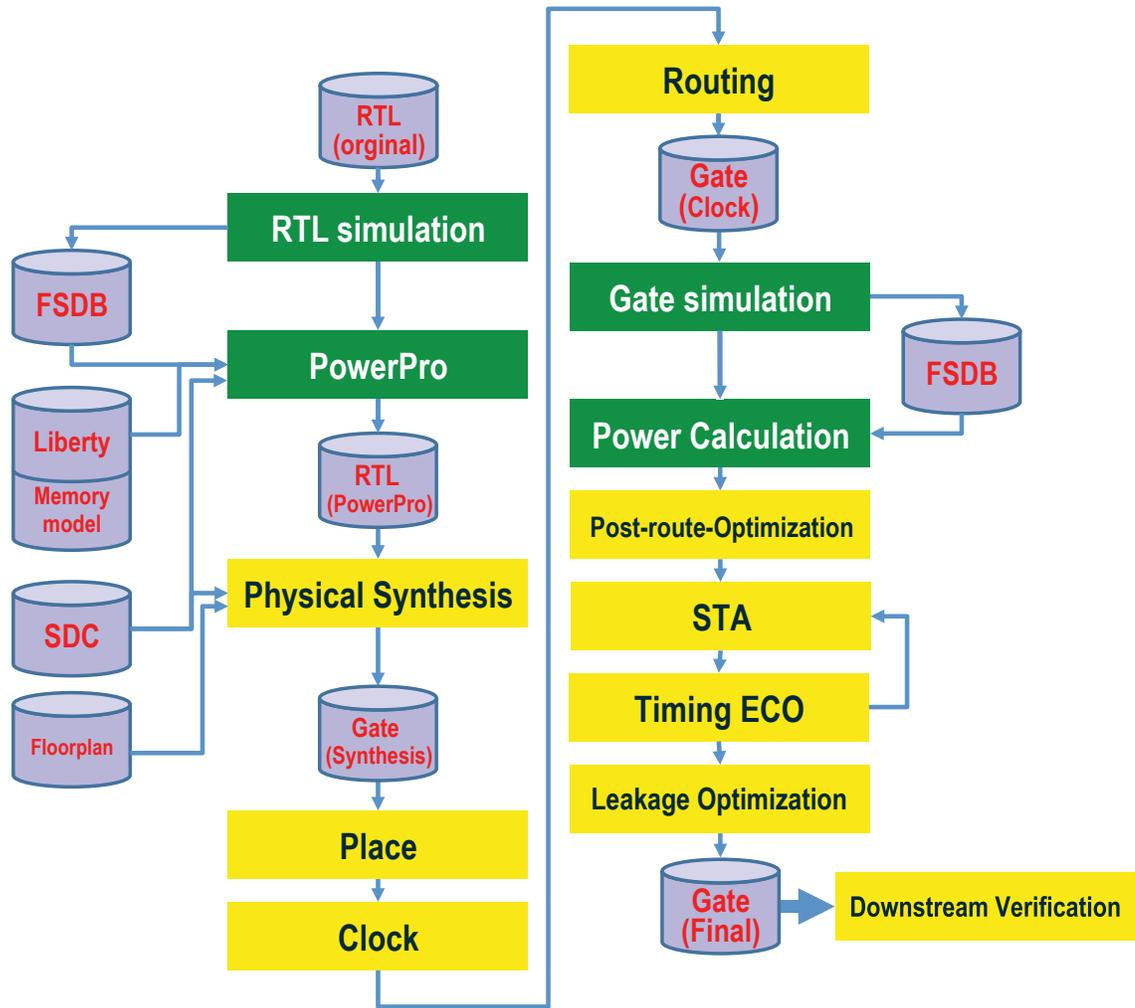
Figure 8: Adding PowerPro to the existing design flow
