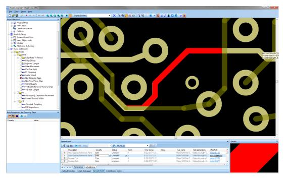
HyperLynx DRC performs electrical Design Rule Checks on boards for EMI/EMC issues, as well as Signal Integrity and Power Integrity. Automated net filtering suppresses false violations.
