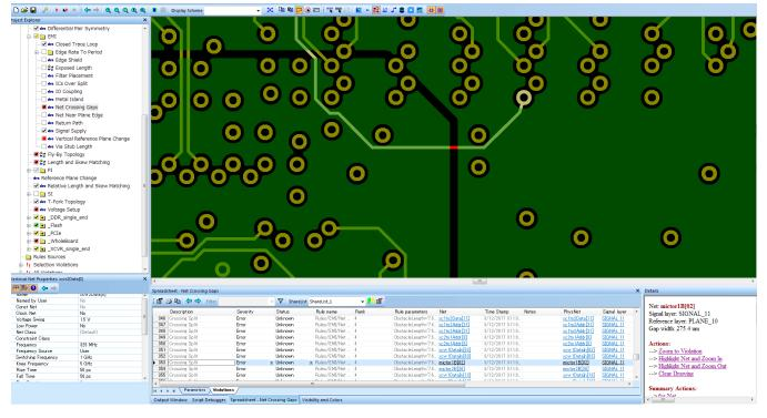
Quickly and easily pinpoint trouble spots that can cause issues on your board with Signal Integrity, Power Integrity, and EMI/EMC. Automated net filtering suppresses false violations.
