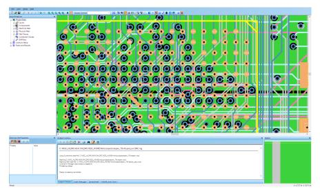
Perform design rule checks on boards for electromagnetic interference and signal integrity issues with HyperLynx DRC.
