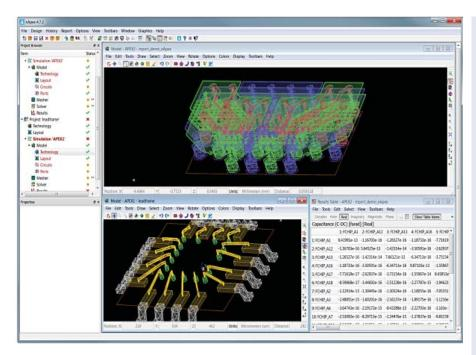
Mentor Graphics HyperLynx Fast 3D Solver is ideally suited for power integrity, low-frequency SSN/SSO, and complete-system SPICE model creation while accounting for skin effect impact on resistance and inductance. The multi-core parallel processing drives extremely fast run times, allowing multiple "what if" scenarios to be run in a minimal amount of time.
