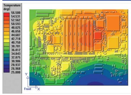
HyperLynx Thermal allows engineers and PCB designers to analyze board-level thermal problems on placed, partially routed, or fully routed PCB designs from all popular PCB layout environments. Temperature profiles, gradients, and excess temperature maps enable designers to resolve board and component overheating early in the design process.
