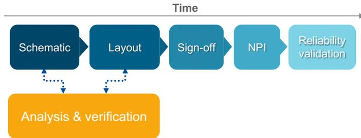
Figure 3 – A Shift-Left Approach for Integrating Verification into the Design Process
